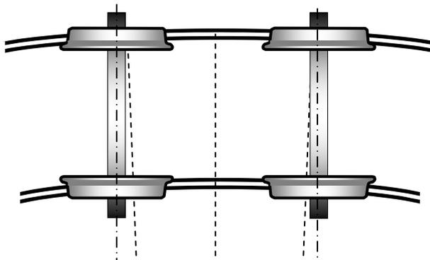
**Fig. 9.31** Bogie in curve.
